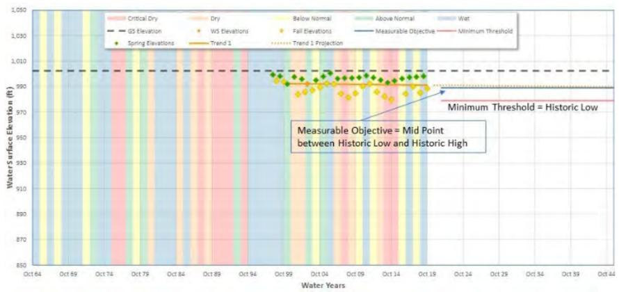
Figure 8-1. Groundwater Level Minimum Thresholds and Measurable Objectives
